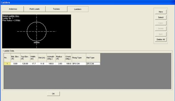
In this window the pole elevation is shown along with the plan cross-section at the bottom of the ladder. To add a new ladder select **New** and a blank line with a rail type, and rung type (none) is shown. The user inputs the following data as defined below:
