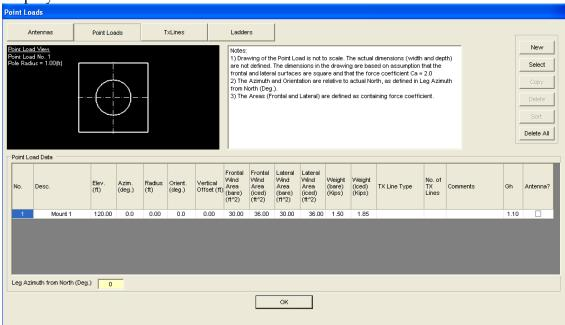
In this window the pole elevation is shown along with the plan cross-section at the point load elevation. To add a new point load select **New** and input line with zero values is shown. The user inputs the following data as defined below:
